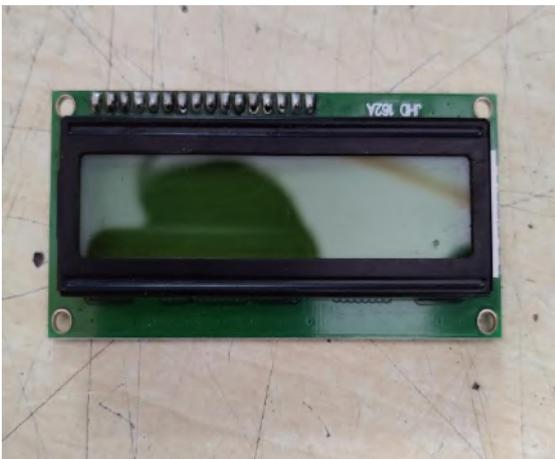
Fig.10: LCD Display
