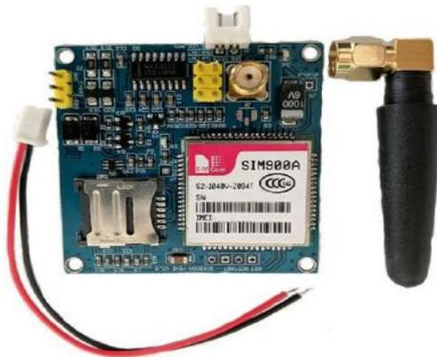
Fig.9: GSM Module
