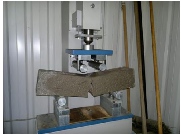
Fig.1- Concrete beam load testing device
