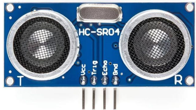
Fig 2: Ultrasonic Sensor (HC-SR04)
