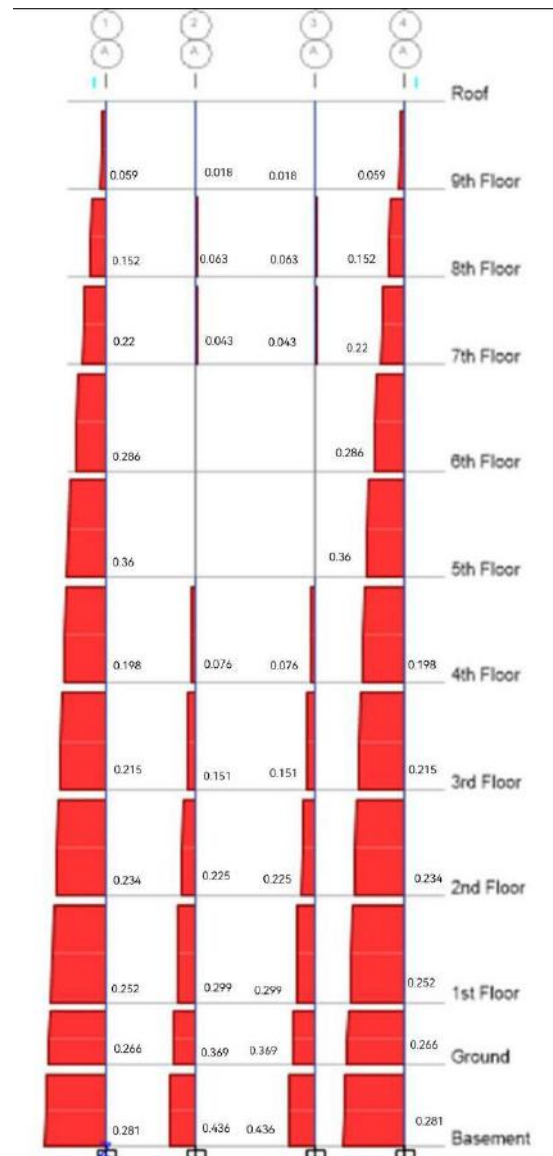
Fig.6: Axial load for columns after columns were removed and DCR values at grid line A
