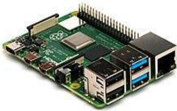
Fig.2: Raspberry Pi Model 4B
