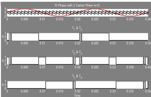
Fig.9: R Phase With Combined Switching Pairs( T_1 & T_2 , T_2 & T_3 , and T_3 & T_4 ) at m=2.0
