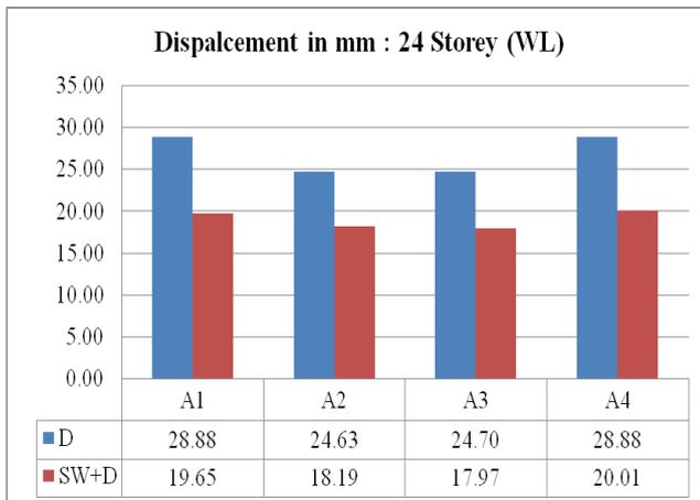
Fig. 10: Maximum Story Displacement in mm 24 Storey
