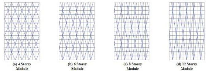
Fig.5: 4, 6, 8 and 12 storey diagrid Module
