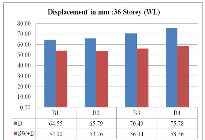
Fig. 12: Maximum Story Displacement in mm 36 Storey
