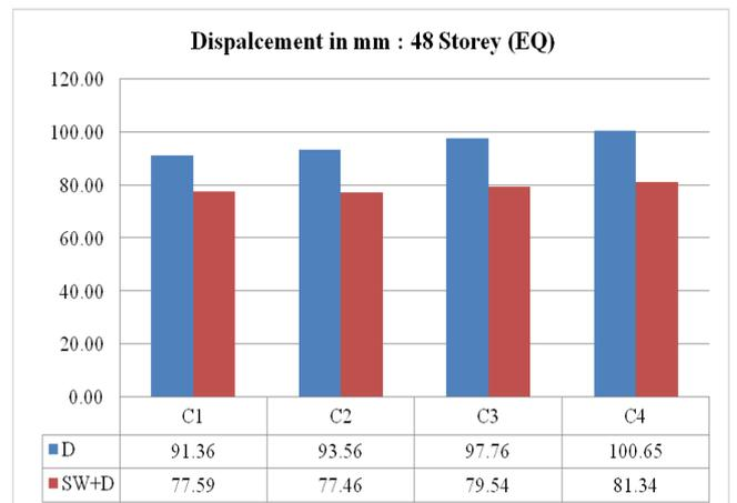
Fig. 13:Maximum Story Displacement in mm 48 Storey
