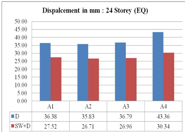
Fig. 9: Maximum Story Displacement in mm 24 Storey
