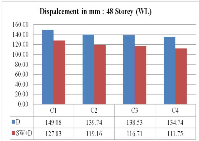
Fig. 14: Maximum Story Displacement in mm 48 Storey
