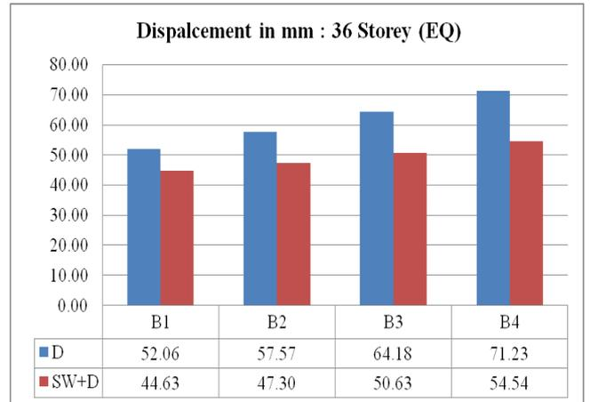
Fig. 11: Maximum Story Displacement in mm 36 Storey
