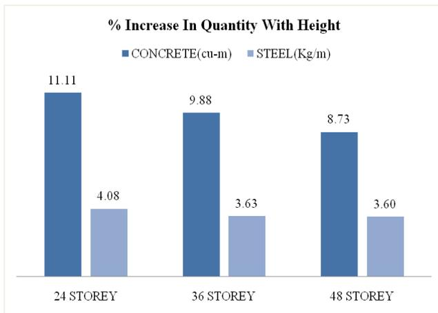
Fig. 24: % Increase In Quantity With Shear Wall
