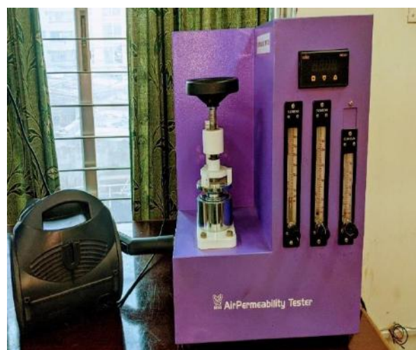
Fig.2 - MAG Air permeability
