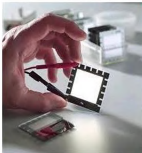
Fig.2: White OLED device for lighting applications. Courtesy of OLED Works.
